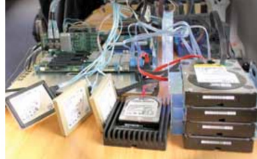
Prototype lab system, incorporating Intel solid state disk technology, used for high speed data capture and stream processing.
